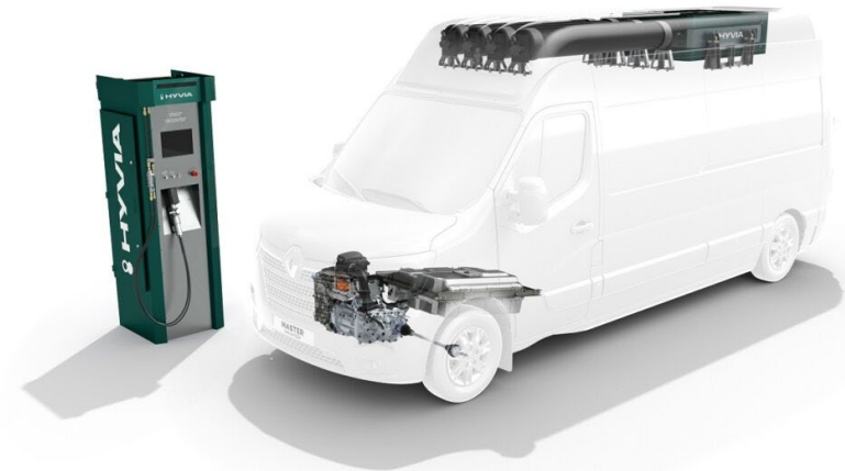
Battery capacity = 33 kWh (around 100 km range) + 6kg H 2 Target : 500 km range
