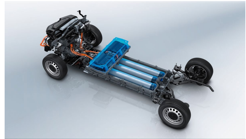
Battery capacity = 10,5 kWh (50 km range) + 4,4 kg H 2 at 700 bar : Target : 400 km range
